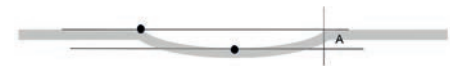
The deformation value is the height difference A between the two points shown
