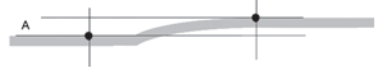
Deformation value is the height difference A between the two points shown.
